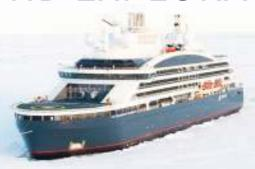
LE COMMANDONT CHARCOT is the first deep polar expedition cruise ship to be equipped with a hybrid liquefield naturall gas (currently the cleanest energy available) propulsion and a bank of high capacity batteries
